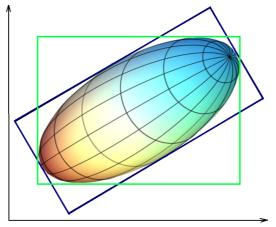
axis-aligned bounding box (AA) shown in green object-oriented bounding box (OO) shown in blue
