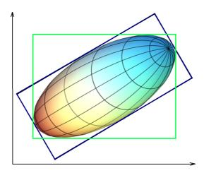
axis-aligned bounding box (AA) shown in green object-oriented bounding box (OO) shown in blue
