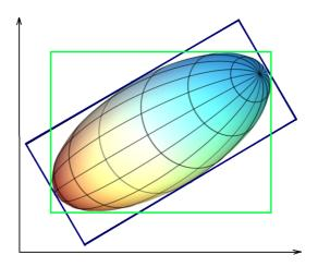
axis-aligned bounding box (AA) shown in green
